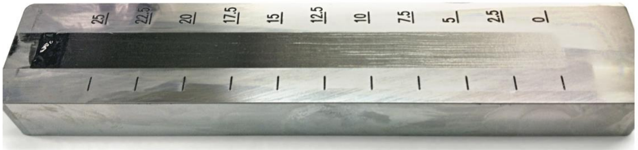
Figure 8. “Good” quality dispersion (particle size \leq 15 \mu\text{m} )
