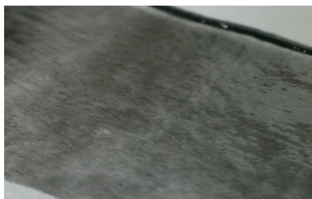
Figure 7. Good quality dispersion (homogeneous mixture)
